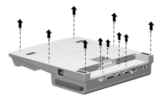
Figure 6-9. Removing the Bottom Cover Screws
